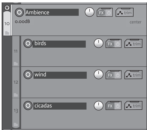
Figure 5.9 Left-clicking the folder icon on the bottom left of Track 10 makes it a folder; it becomes a parent track, with tracks 11–13 here now its children. Clicking the folder icon again restores the child tracks to normal.
