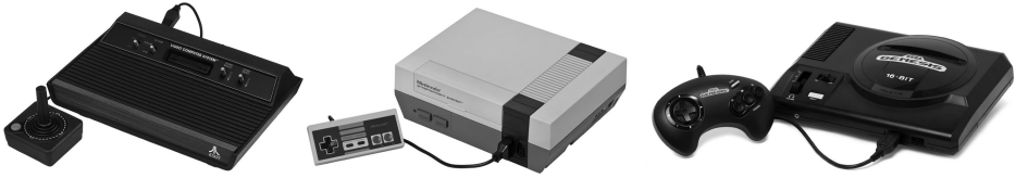
Figure 1.4 Home consoles through the years: The Atari 2600 (1977, left), the Nintendo Entertainment System (1985, center), and the SEGA Genesis (1989, right), each with increasing levels of sonic sophistication: two channels, five channels, and ten channels of audio, respectively (Evan-Amos/Public domain).
