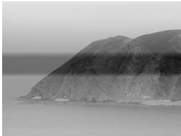
Figure 5-27 Rolling bars distortion.
